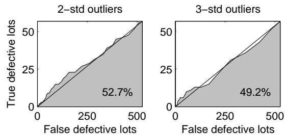
Figure 1: ROC curves corresponding to the number of 2-std and 3-std outliers in all in-fab tests for a specific lot. A test result is considered to be a k -std outlier if its value is more than k standard deviations from the expected result of the test.
